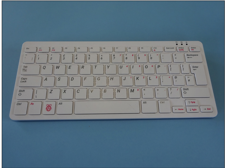
FIGURE 1-3: The Raspberry Pi 400 hides the computer inside the keyboard.
